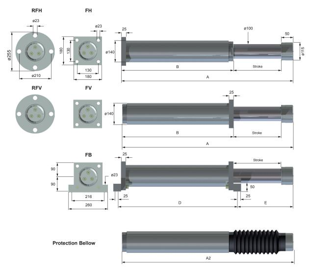
Rear flange recommended only for shock absorbers up to 300 mm stroke!
