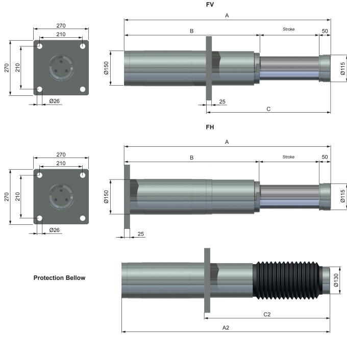
Rear flange recommended only for shock absorbers up to 300 mm stroke!
