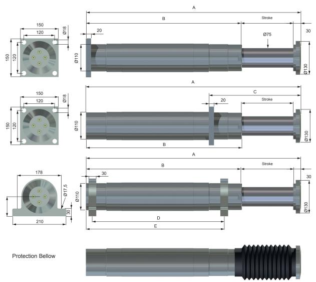
Rear flange recommended only for shock absorbers up to 300 mm stroke!
