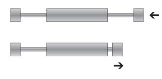
Double-acting with spring return As one piston rod travels in, the opposite rod remains out
