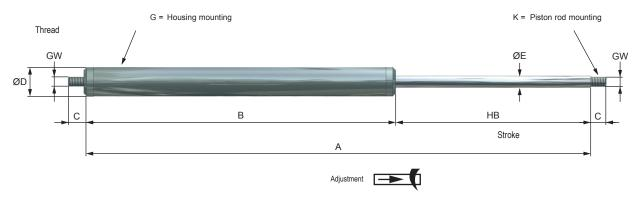
Design ZG without return stroke with volume compensation of piston rod through floating piston. Return force, see table Installation position: any position
